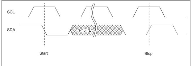
Note : At the write operation, the FRAM device does not need the programming wait time (twc) after issuing the Stop Condition.
