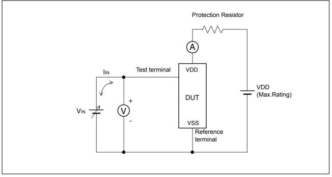
Note : The voltage V<sub>IN</sub> is increased gradually and the current I<sub>IN</sub> of 300 mA at maximum shall flow. Confirm the latch up does not occur under I<sub>IN</sub> = ± 300 mA. In case the specific requirement is specified for I/O and I<sub>IN</sub> cannot be 300 mA, the voltage shall be increased to the level that meets the specific requirement. · C-V method of Latch-Up Resistance Test
